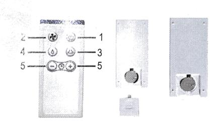
To replace the battery, slide the back panel of the remote-control down to release it. Remove old battery and replace with CR 2025 round battery.
