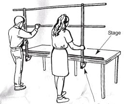
Lift the Lower Bracket on each Upright until the Tee Handle drops down.
