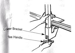
Place the Guard Rail onto the Stage with the Lower Bracket on each Upright positioned below the deck surface as shown at the right.
