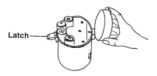
2. Remove the two battery containers and take out any old batteries. Install four batteries in each container, as indicated by the diagrams on the containers.
