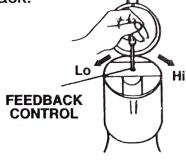
Note: Adjusting the FEEDBACK CONTROL also reduces the volume. To increase the volume, rotate the FEEDBACK CONTROL clockwise until the sound is audible without feedback. If you are unsure how to make this adjustment, have a professional electronics technician adjust it for you.
