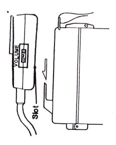
3. Make sure the TALK button on the left side of the microphone is not in the LOCK position, since this disables the TALK button on the megaphone's handle.
